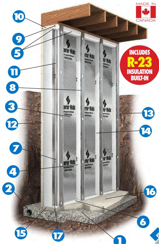
**Special Note:** Items #1,2,&16 as well as the joist/flooring system are provided on site per Superior Walls specifications by builder and contractors as an integral part of the Superior Walls foundation system.
